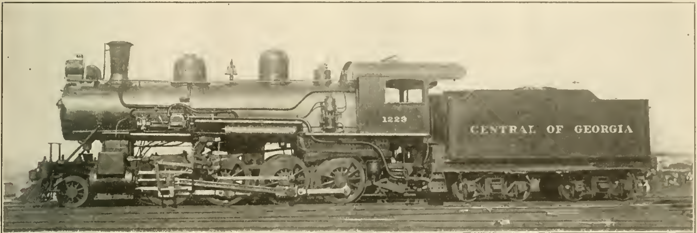
CONSOLIDATION WITH FEED WATER HEATER ON THE CENTRAL OF GEORGIA RAILWAY.
